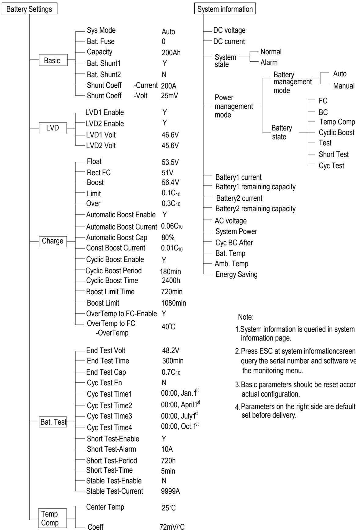
Figure 11 Menu structure of the battery parameter
