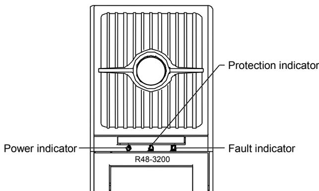
Figure 1 Front panel of the rectifier
