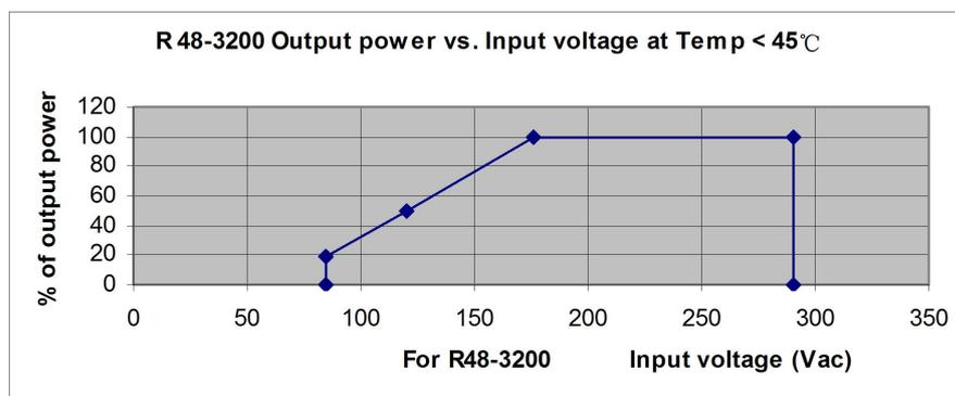
Figure 3 Relationship between output power and input voltage of the rectifier (the temperature is less than 45°C)
