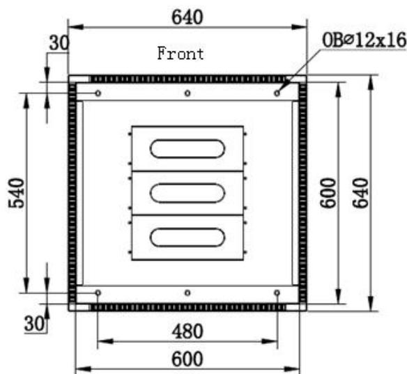
Figure 2-1 Installation size of the cabinet base (unit: mm)
