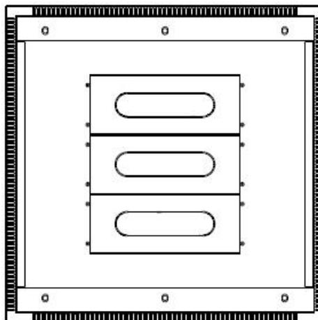
Figure 2-6 Position of the rubber cable entry hole
