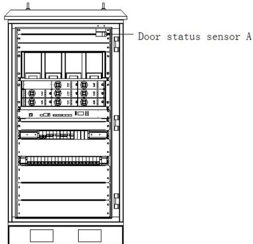
Figure 5-5 Position of the door status sensor
