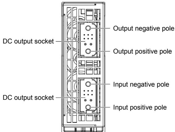
Figure 7 Rear panel of the solar module
