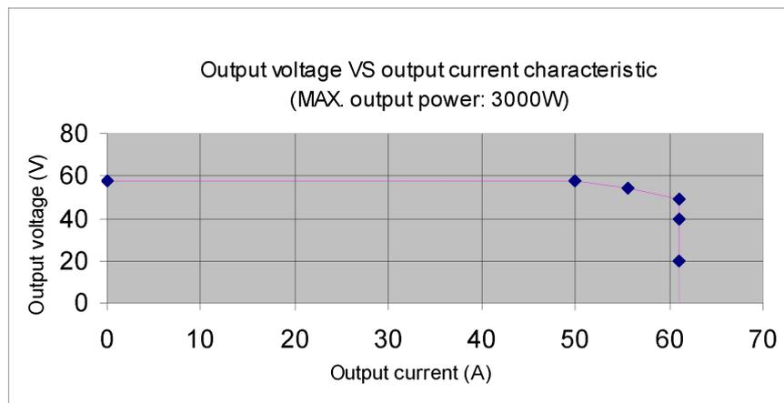
Figure 8 Schematic diagram of the relationship between output voltage VS. output current (the solar module outputs 3000W)
