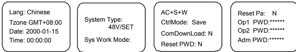
Figure 4-44 System parameter setting screen
