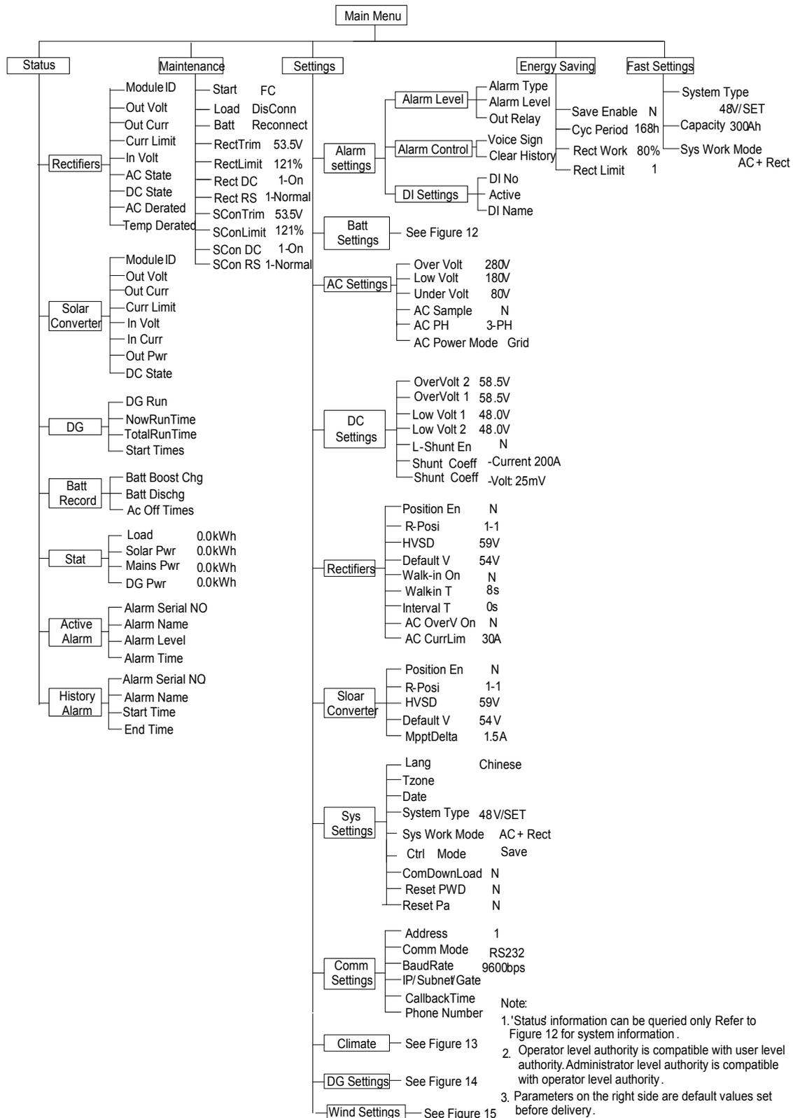
Figure 10 Menu structure of the controller
