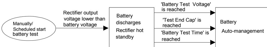
Figure 4-33 Schematic diagram of the test function
