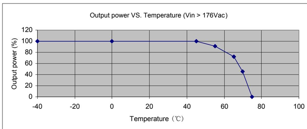
Figure 5 Schematic diagram of the relationship between the output power and ambient temperature of the rectifier
