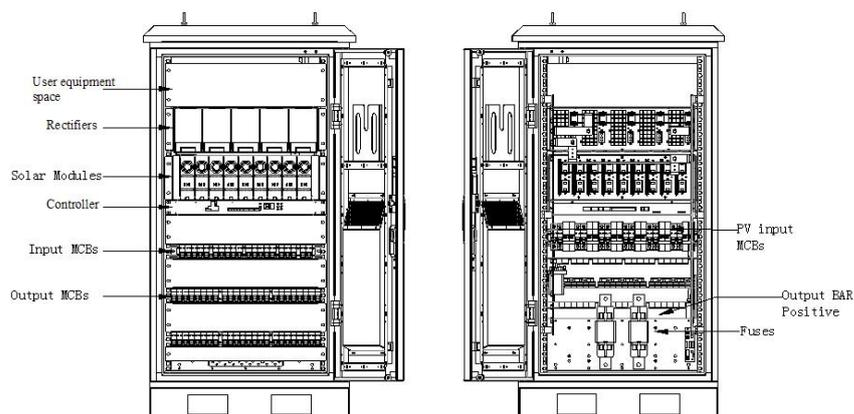
Figure 1-2 Structure diagram
