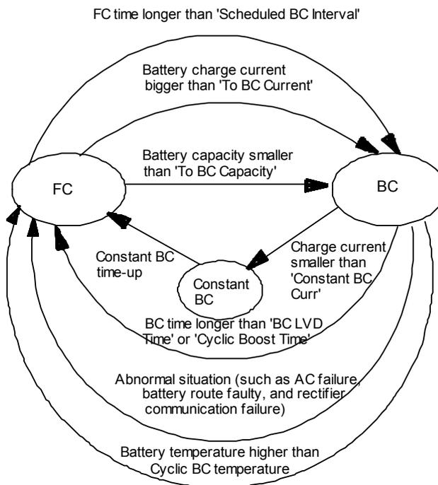
Figure 4-31 BC/FC switchover diagram
