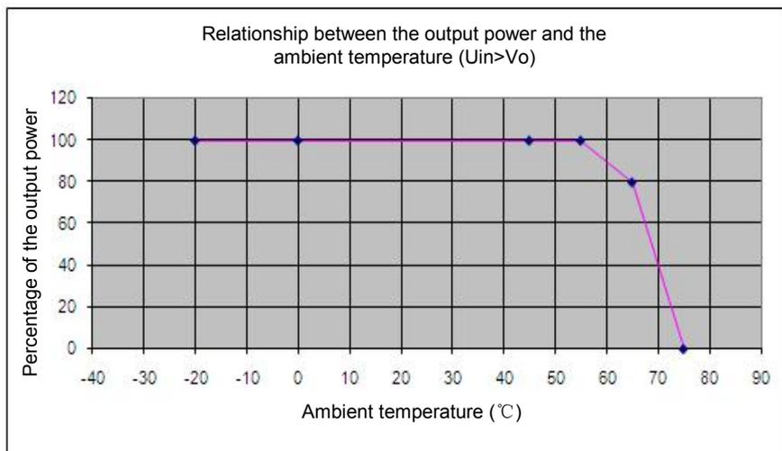
Figure 9 Relationship between output power and ambient temperature of the solar module
