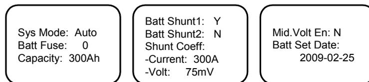
Figure 4-28 Battery basic parameter setting screen
