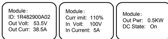
Figure 4-16 The information screen of the solar module
