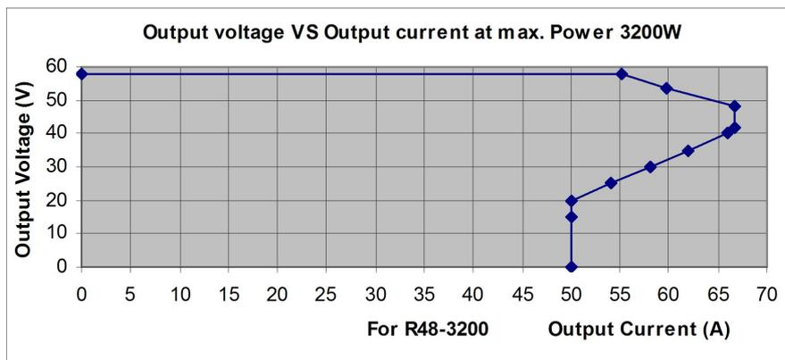
Figure 4 Schematic diagram of the relationship between output voltage and output current with the rectifier outputting 3200W
