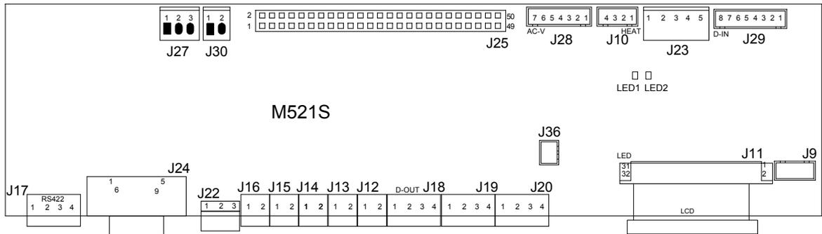
Figure 5-4 Indicators and ports of the M521S monitoring board
