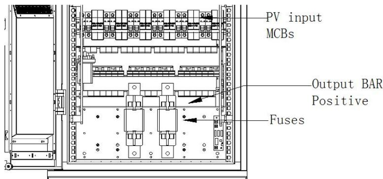
Figure 2-9 System power distribution unit Front View
