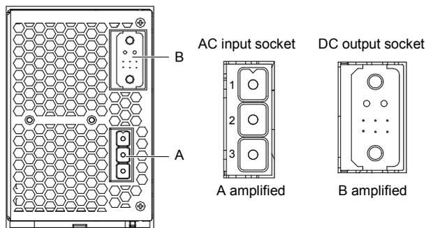
Figure 2 Rear panel of the rectifier
